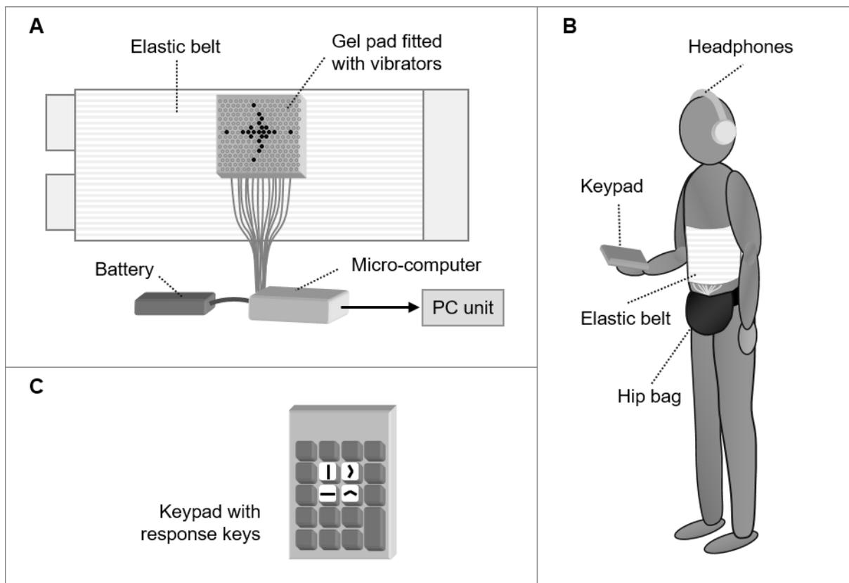
*Note.* Panel A: Apparatus. Panel B: Equipment. Panel C: Response keypad.
